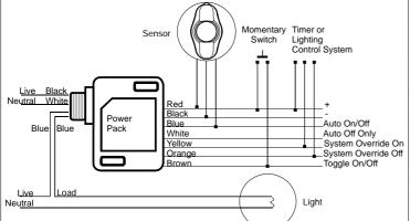
[Blue] Automatically turn light on/off based upon presence detected by an occupancy sensor.
